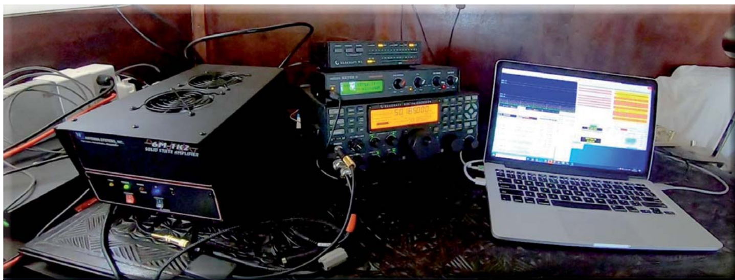
6 m EME station – M2 Systems M6-1K2 Linear, Elecraft K3S, Elecraft W2 Watt Meter Eltek 2 kW 50 V Power Supply, Microham Keyer II and MacBook Pro
