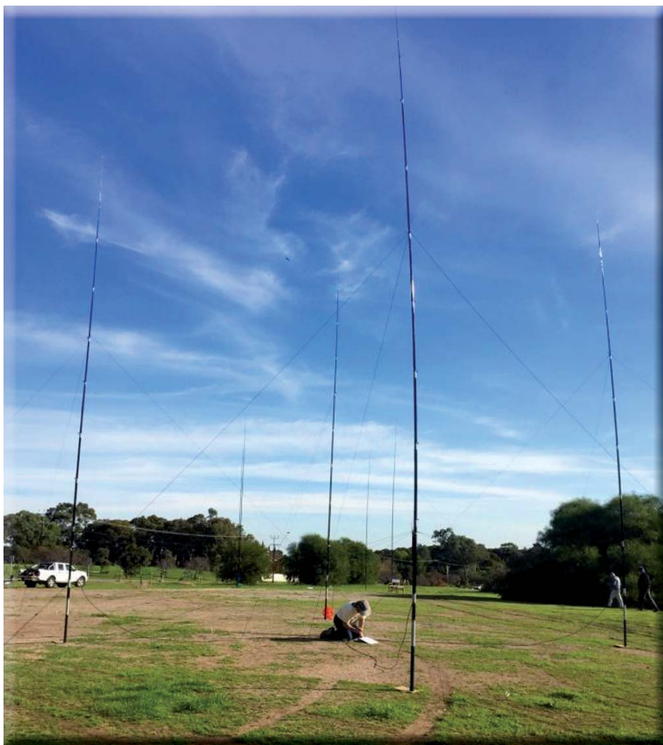
Tune & Test Day in Adelaide 30 and 40 m 4-square arrays
