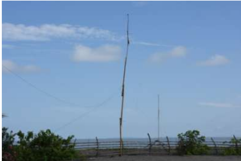
3 element 20 m band Vertical Dipole Array (eco friendly version)
