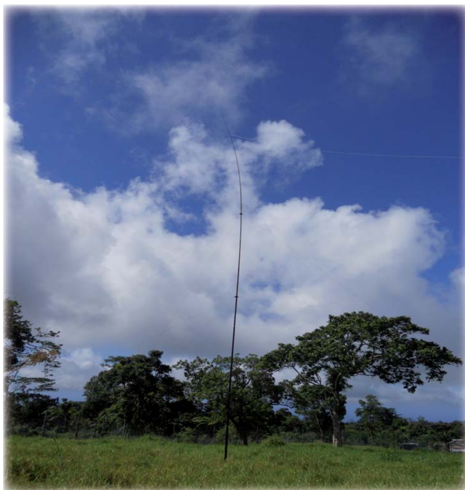
5WØGC's vertical antenna on 160/80/40 m during a storm
