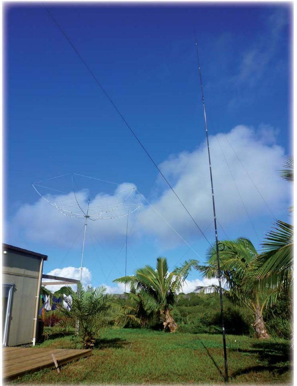
Hexbeam with 30 m and 160 m vertical at background
