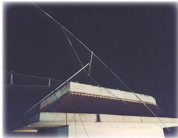
TL8AO broken beam
