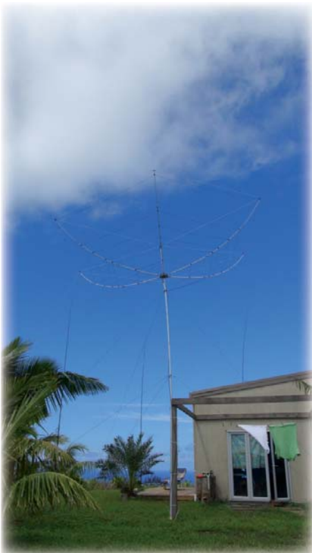
Hexbeam with 30 m and 17 cm Vertical
