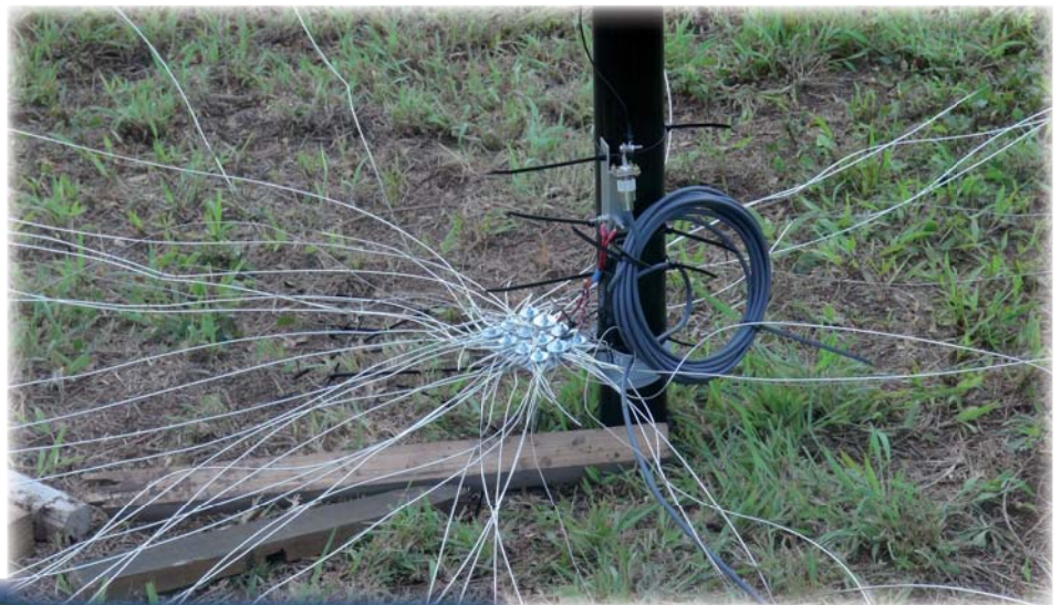
Base of 160 meter inverted-L
