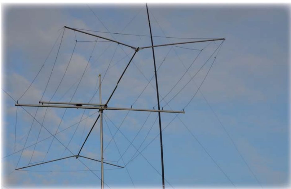
XX9D – LZAW 10-5 Antenna for 20 and 10 m Band
